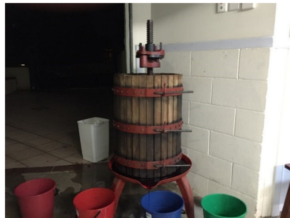
Figure 8 – A wine press is used to separate the juice from the skin. Almost like a fine-screen at a treatment plant.
