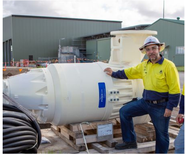
Figure 12: These are the type of pumps that I tend to work with (this pump has a capacity of 950 L/s)
